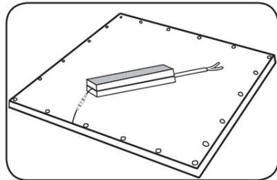
2 Umieść zasilacz na tyle panelu. / Place the driver on the back of the panel.
